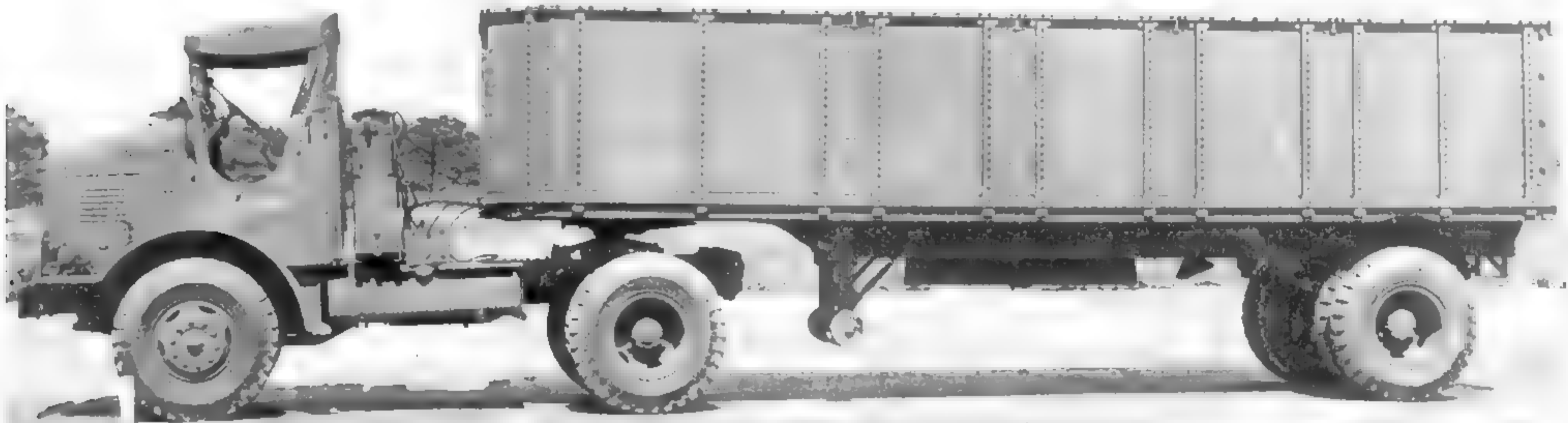
This photo, taken in June 1944, shows an International Harvester M425 doing what it was built for — towing a 25-ft., 10-ton semi-trailer. Hundreds of similar combinations were used by the famed Red Ball Express. (U.S. Army photo)
